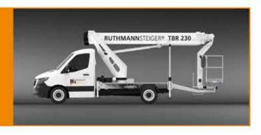
4 movements simultaneously possible (lift, rotate, telescope, Rüssel up/ down) + basket rotation
