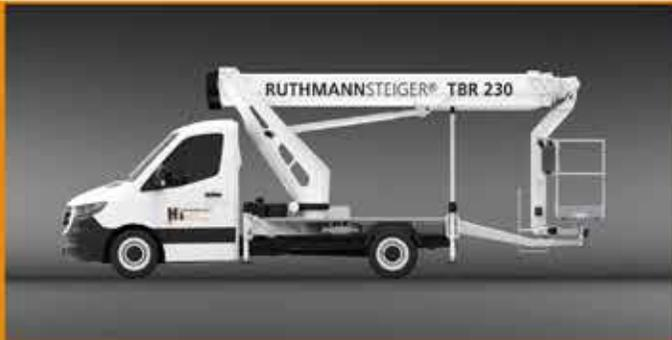
4 movements simultaneously possible (lift, rotate, telescope, Rüssel up/down) + basket rotation
